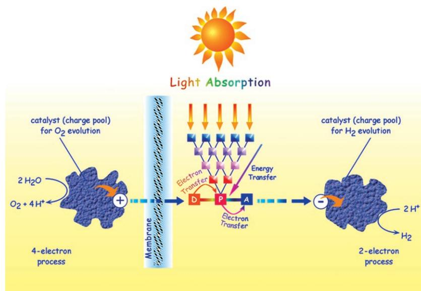
**Figure 8.** A very simplified sketch representing key processes in artificial photosynthesis: solar light harvesting by molecular antennas, energy transfer to a reaction center, charge separation, water splitting with production of hydrogen and oxygen on the two sides of a membrane (adapted from ref [37]).
